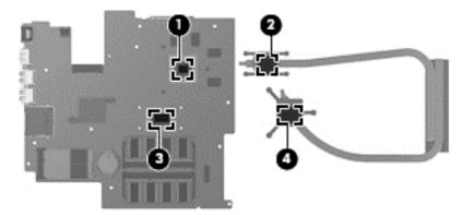
c. Loosen the captive screws (1) and lift the UMA graphics heat sink (2) from the system board.
